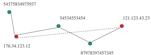
Once a message gets from the node 543... to the node 176.34.123.12, then this is able to create a direct connection to the source, shorting up the overall hops number.
